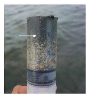
Figure 2. Sediment corer used to quantify oxygen penetration depth. Consistently darker sediment indicates anoxic sediment, as indicated by a white arrow.
